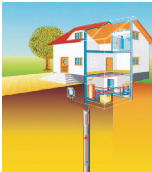
Fig. 8.29. Vertical borehole heat exchanger system; yellow box in building basement: heat pump [99Ano1].
