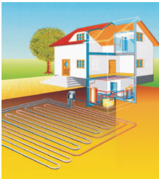
Fig. 8.28. Horizontal Earth coupled heat exchanger system; yellow box in building basement: heat pump [99Ano1].
