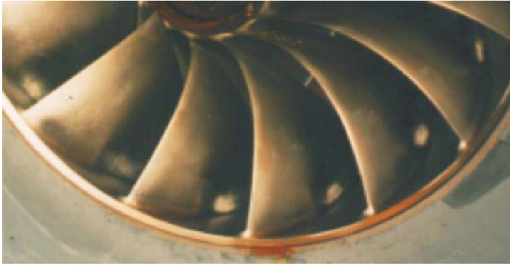
Fig. 2.2.13. Cavitation erosion on a turbine runner.
