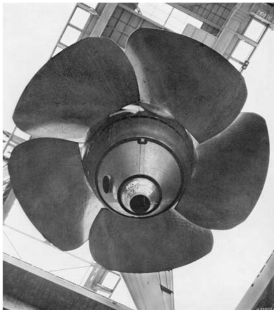
Fig. 2.7.16. Kaplan runner with a diameter of 8.4 m and 5 blades (Aschach, Austria, P_{\max} = 75 MW) [ VSH ].
