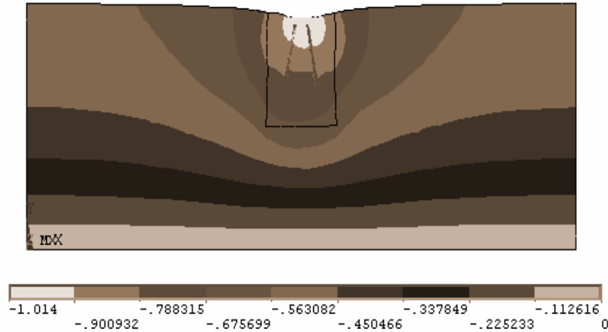
Figure 3. Settlement of soil for state that soil is loaded under maximum load (900 Kpa).
