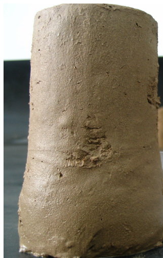
(a) Sample after liquefaction test
