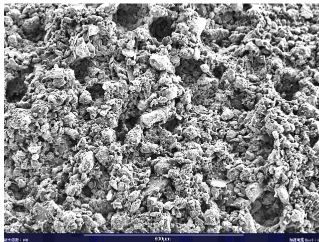
(b) Microstructure feature after liquefaction (Magnification factor 100)
