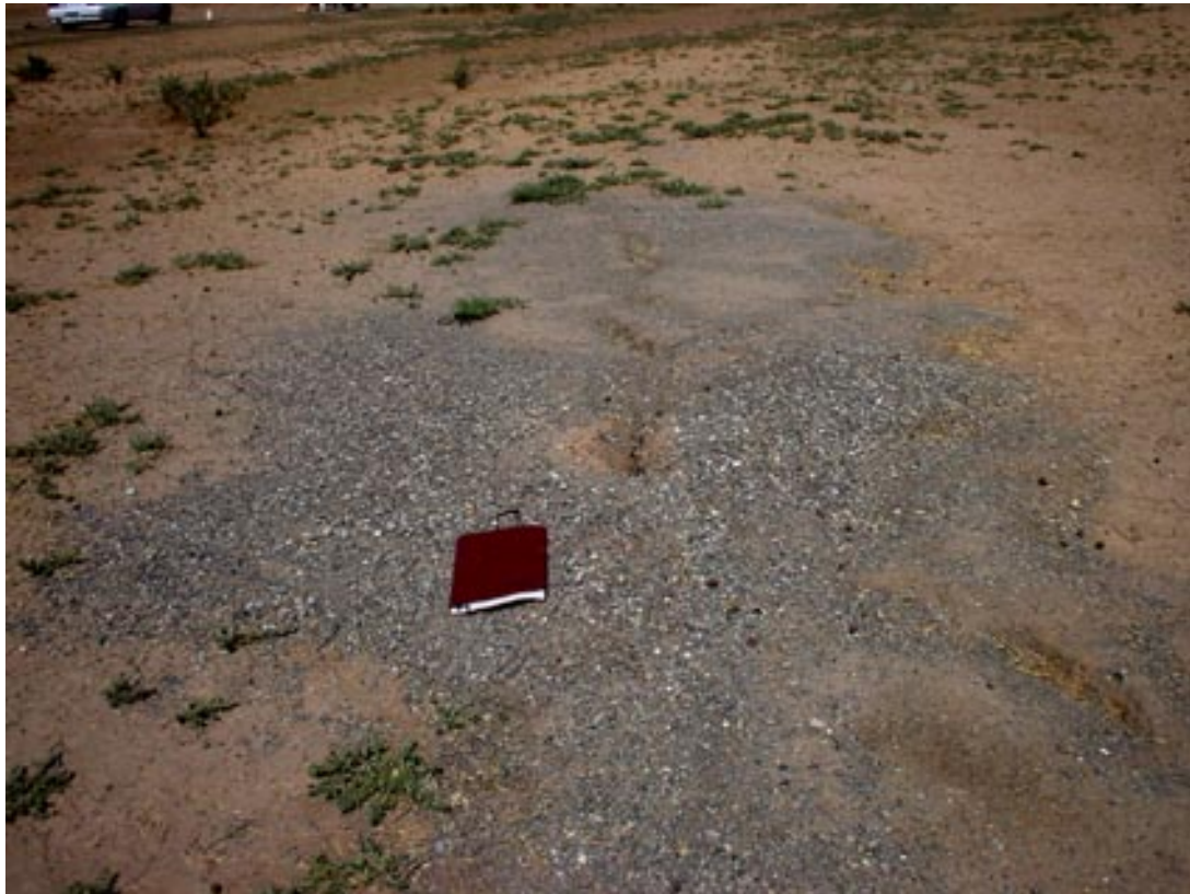
Figure 3. Liquefied gravel at point B
