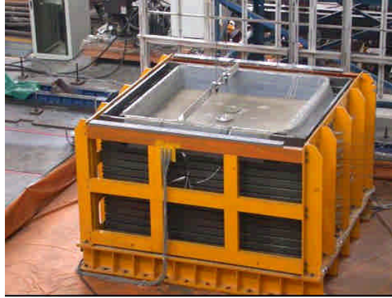
Figure 1. Large biaxial laminar shear box on shaking table at NCEE
