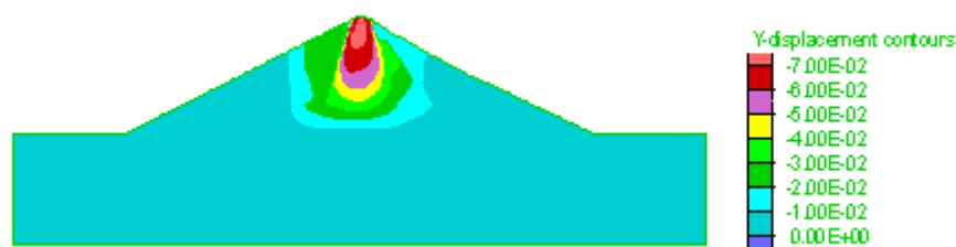
Figure 2. Contour of y-directional displacement induced by material dam construction.
