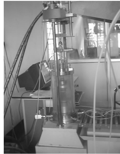
Figure 5. Cyclic Triaxial Testing Machine
