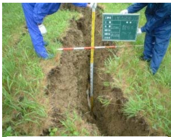
Figure 5. Crack on land side at Kimazuka
