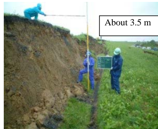
Figure 4. Difference in level at Kimazuka
