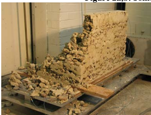
Figure 2c,d: Collapse at 0.32g
