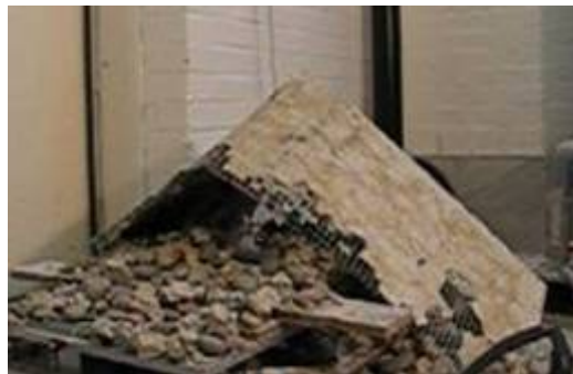
Figure 8 Failure mechanism at 1.02g of Test C with wire mesh reinforcement
