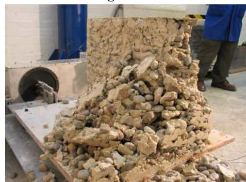
Figure 2c,d: Collapse at 0.32g
