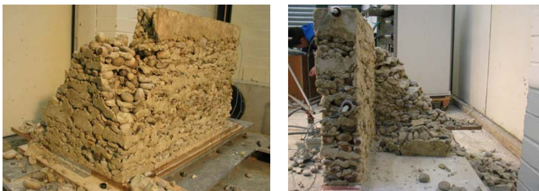
Figure 4: Failure at 0.32g
