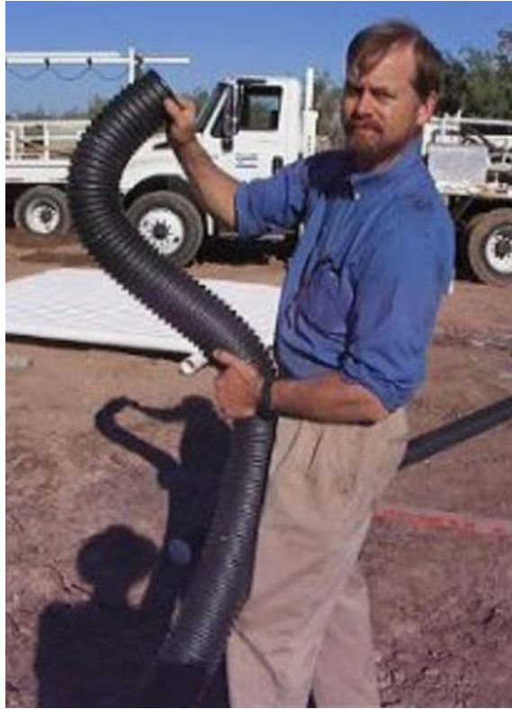
Figure 11. Demonstration of flexibility of corrugated drain pipe installed for future survey of lateral ground displacement versus depth through liquefiable layer
