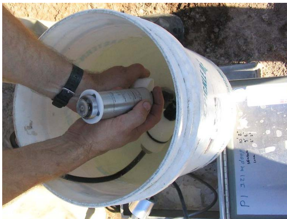
Figure 9. Pressure transducer, sensing element upward without filter, being saturated in bucket of water in preparation for installing the assembly in casing below the bucket
