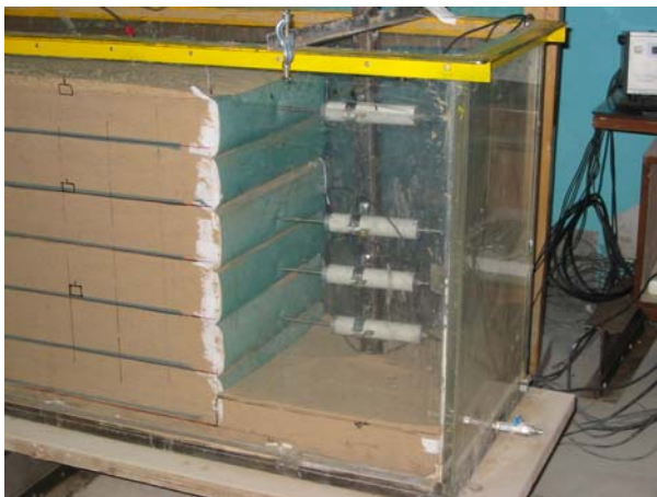
Figure1. A typical reinforced earth model wall with wrapped geogrid facing
