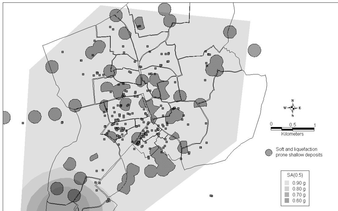
Figure 12. Variation of spectral acceleration corresponding to 0.5 s period (squares indicate locations of collapsed buildings and dark gray patches mark the soft sites)
