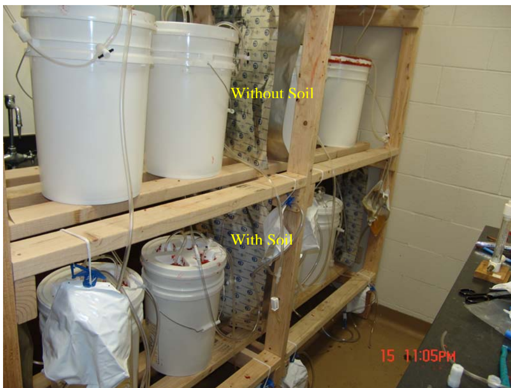
Figure 2 Two sets of bioreactor cells with and without soil representing the four phases of decomposition
