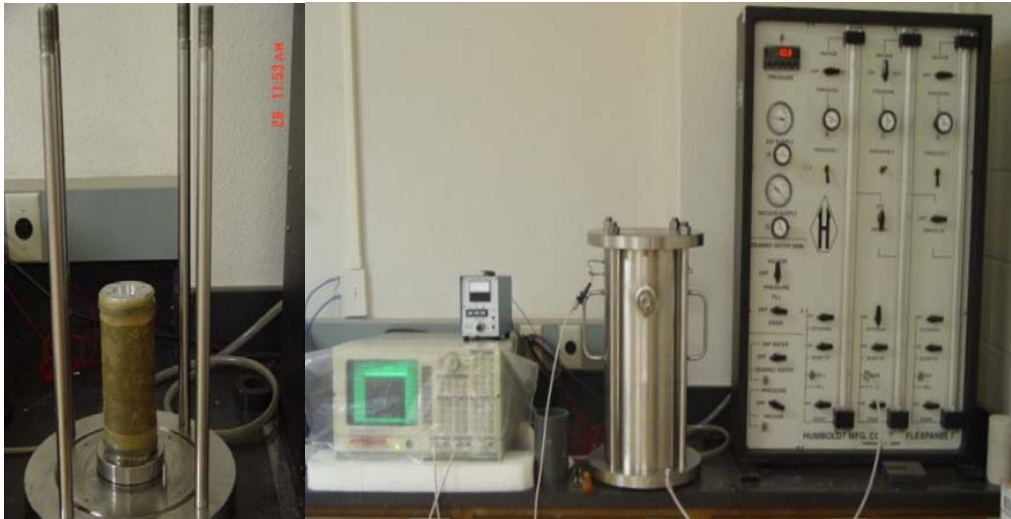
Figure 5 Resonant column test setup with a 71 mm. diameter solid waste sample
