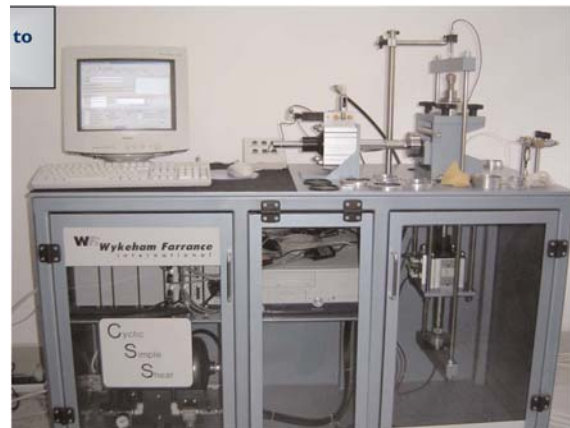
Figure 3- NGI-type direct simple shear device at Soil Dynamics Laboratory of the Sharif University
