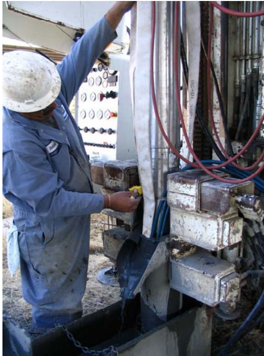
Figure 5. Using the drill rig to lower the DFSD into the mud filled casing. Note flat white hoses for clamping, thinner blue hoses supplying water, and the large hydraulic clamps holding the casing in place.
