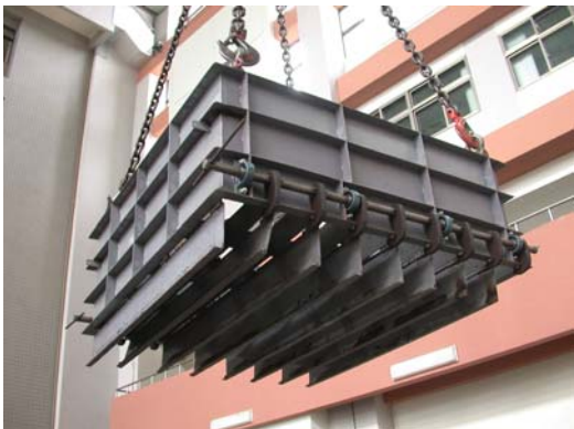
Figure 4. The picture of the pluviator
