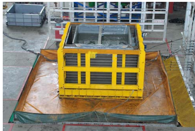
Figure 7. Mailiao silty sand specimen in the shear box on the shaking table
