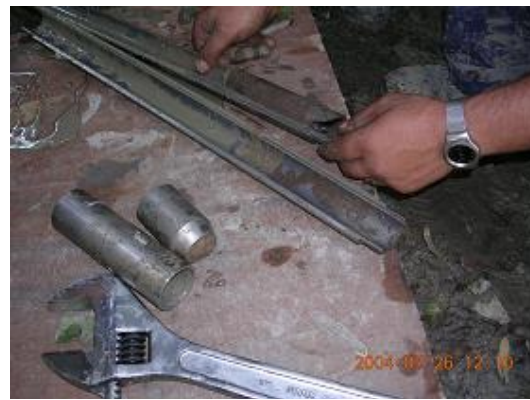
Figure 4. Soil sampling using SPT
