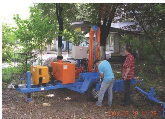
Figure 6. CPT equipment
