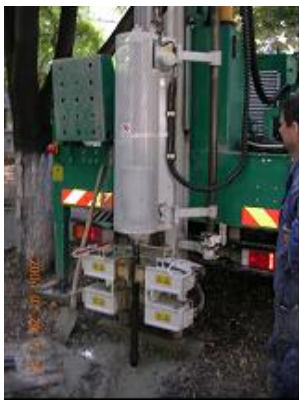
Figure 3. Standard Penetration equipment
