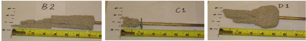
Figure 6. Photographs of excavated grouted piers.
