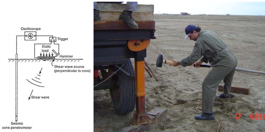
Figure 5. Principles of the seismic cone survey technique [1]
