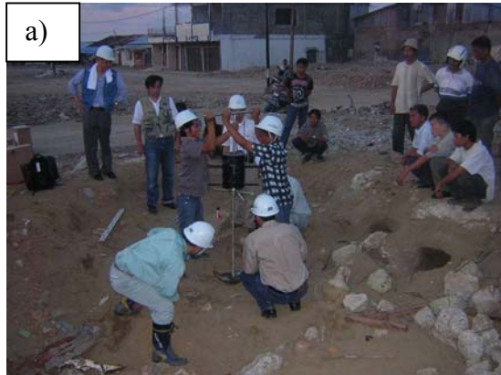
Figure 10. Training on Swedish Weight Sounding Test at (a) Gunung Sitoli b) Idano Gawo Br.)
