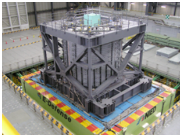
Photo 1 Test model on large shaking table
