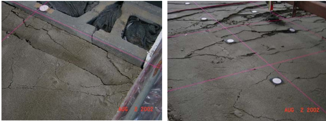
Figure 4. Cracks Behind The Blocks (Left) and In The Backfill Behind Reinforced Zone (Right)
