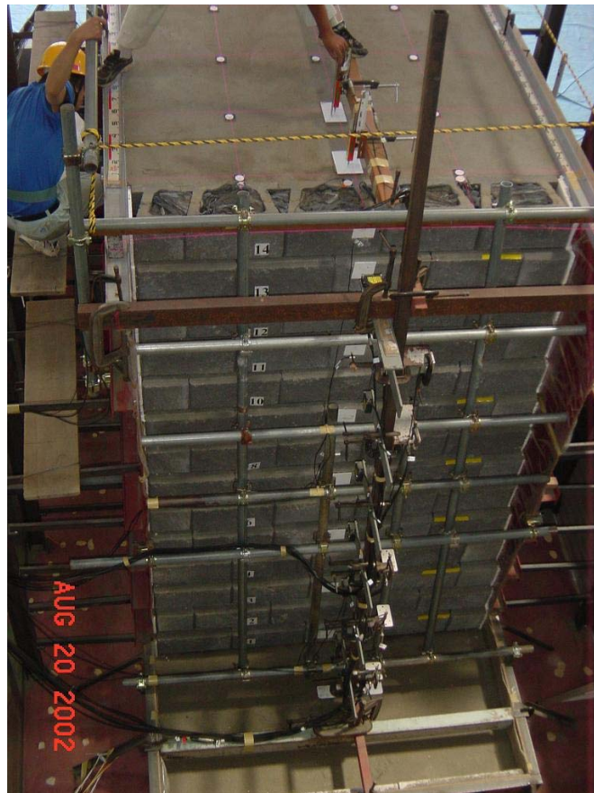
Figure 3. The Wall at End of Construction
