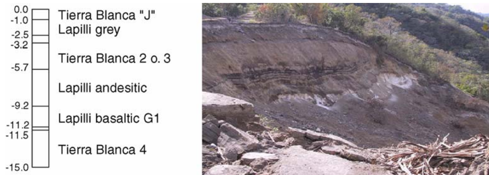
Figure 4. Soil profile (Jibson & Crone, 2001) and picture of the slip zone (Konagai, 2001) at the head of the slope
