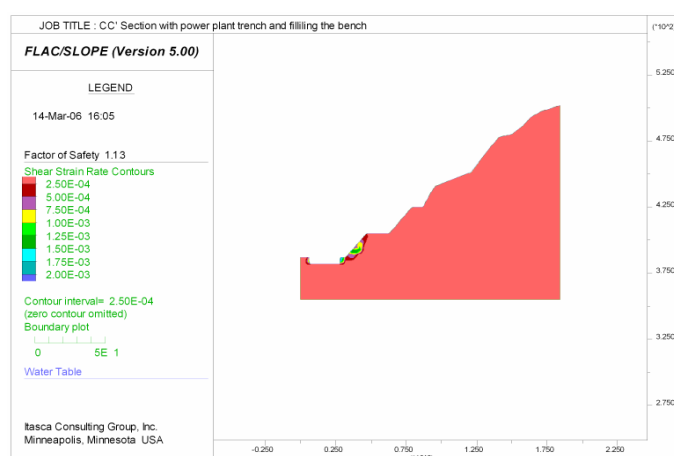
Figure 6. Shear strain rate for saturated state with modified slope's toe, [SF=1.13]
