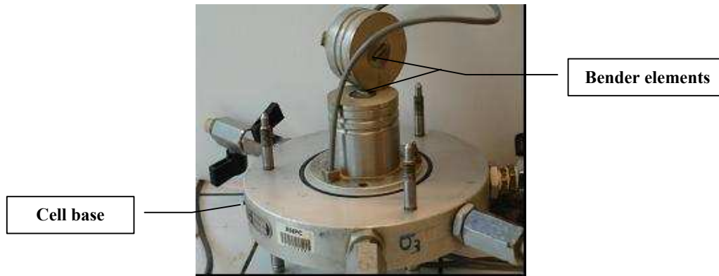
Figure 1. Schematic view of a triaxial cell equipped with bender elements
