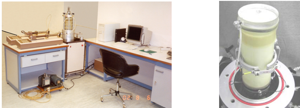
Figure 3. (a) The triaxial (cyclic/monotonic) loading system used in the laboratory program, (b) the local strain measuring transducers used in the triaxial tests on EPS specimens
