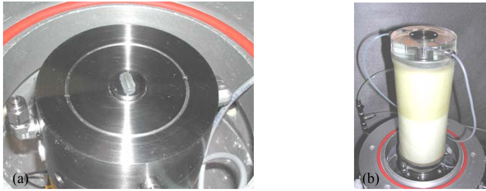
Figure 5. The bender-extender system used in the laboratory program (a) the pedestal of the device with the insert element, (b) EPS specimen mounted in the testing system
