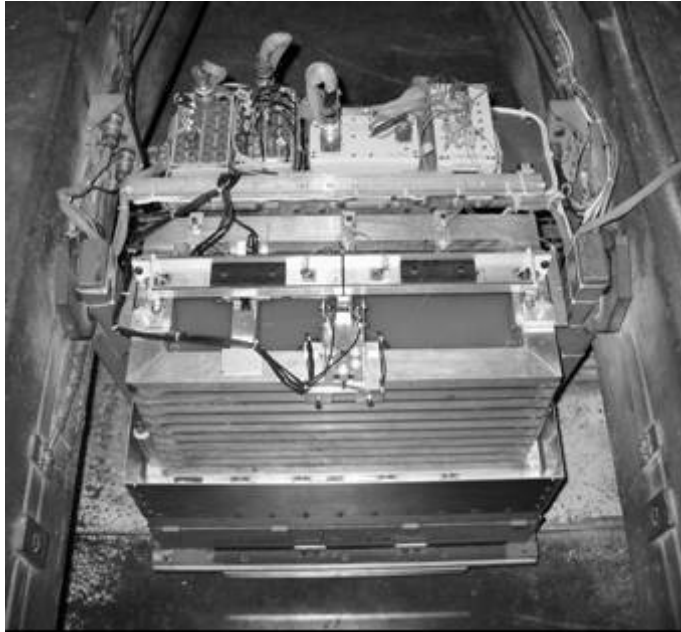
a) model placed in the arm of CUED's beam centrifuge
