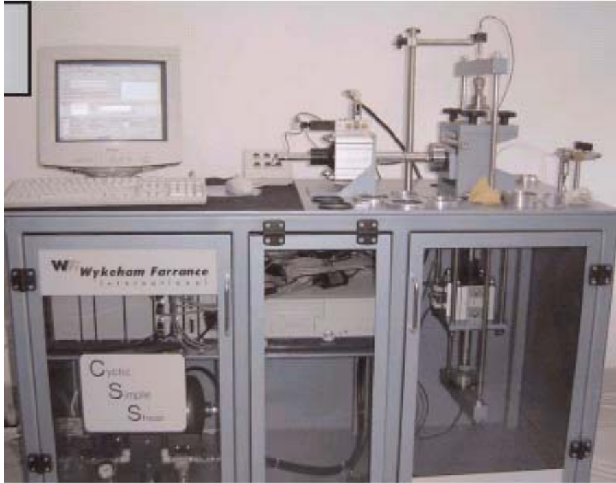
Figure 5. SGI-type cyclic simple shear device at the Advanced Soil Mechanics Laboratory of Sharif University of Technology
