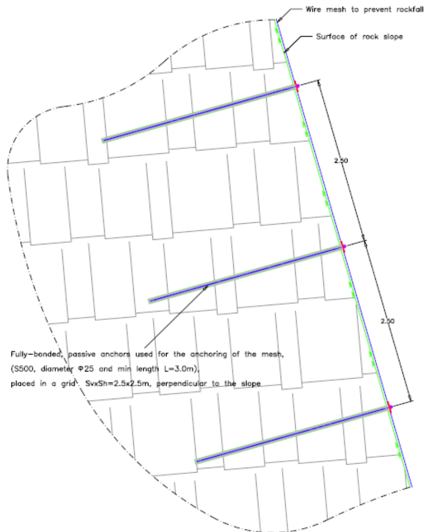
Figure 5 Cross section of rockmass protected by wire mesh kept in place by a grid 2.5x2.5m of 3m length rock bolts, fully bonded into the rockmass
