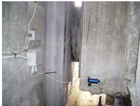
Figure 10. Displacement (transverse) and side load cell
