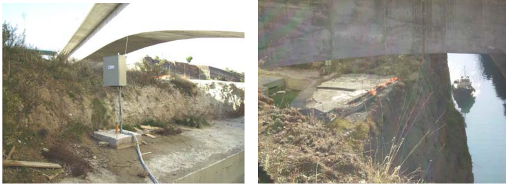
Figure 7. Inclinometers in Isthmus slopes
