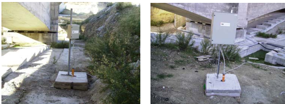
Figure 6. Inclinometers with Data Loggers
