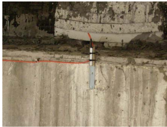
Figure 12. Temperature sensor
