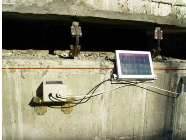
Figure 9. Accelerometer on pier
