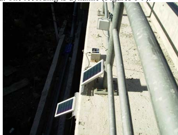
Figure 8. Accelerometer on deck with sun cells
