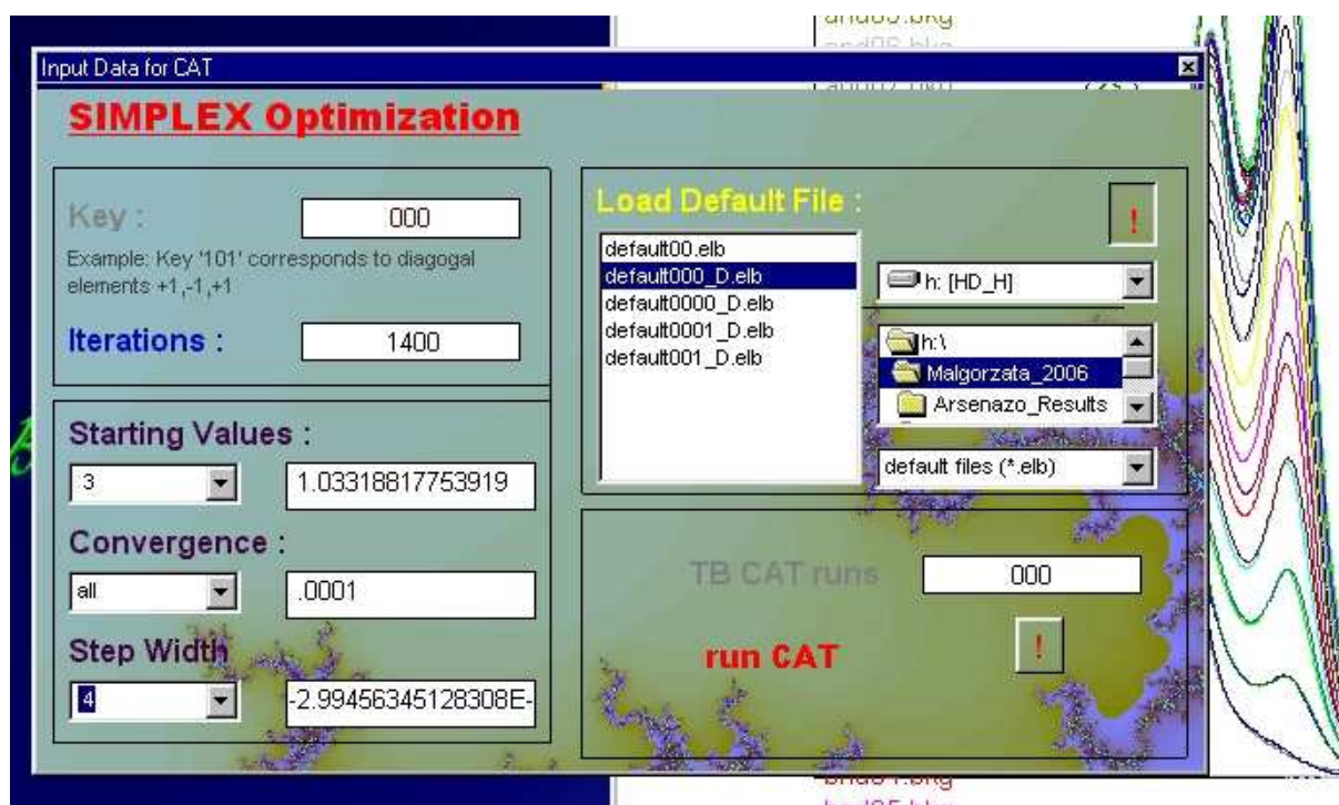
Figure p: CAT input window. The default file default000.elb has already been loaded and the number of iterations is set to 1000. In the next step, the concentration information file example.dat will be loaded. The values from the default000_D.elb file have been copied to the lower left hand side fields with caption 'Starting Values', 'Step Width' and 'Convergence'. These fields can be manipulated by the user.
