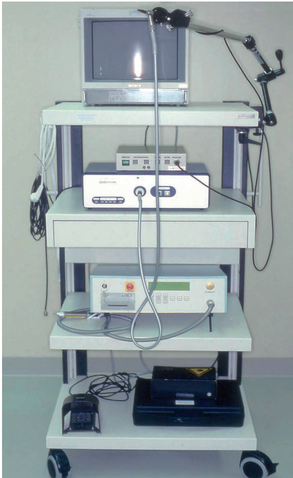
Fig. 10.1. Endoscopic system, featuring monitor, camera, xenon light source, Erbium-YAG laser, and video recorder
