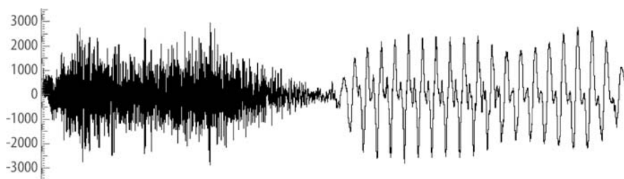
Figure 14.17. Example for a diphone. It shows the right half of the fricative sound [f] and the left half of the vowel [u] from the English word beautiful which was pronounced by a female native speaker. The diphone length is approximately 200 ms
