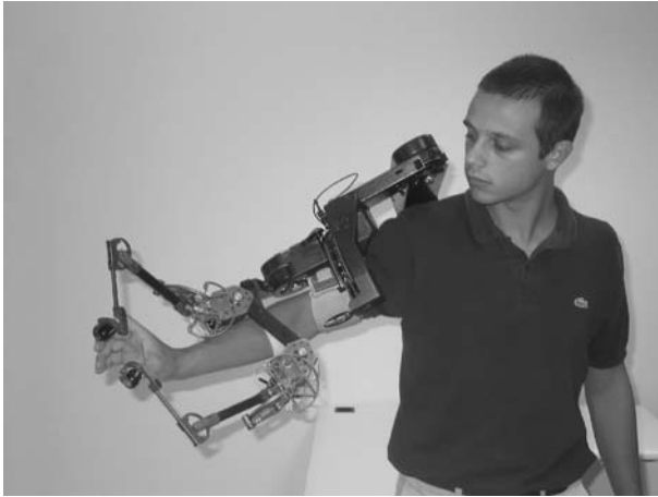
Figure 4.9. The Pure-Form display carried by a user. Image copyright Antonio Frisoli, Massimo Bergamasco, PERCRO, Scuola Superiore Sant'Anna, Pisa, Italy and used by permission
