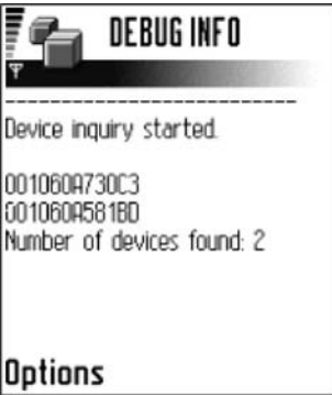
Figure 11.11. Screenshot of bus commuter mobile phone that displays the results of the Device Discovery process
