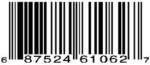
Figure 17.3. Example of a UPC bar code
