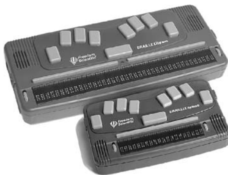
Figure 12.17. Braille notetakers (photograph of the Braille Lite Millennium 20 and 40 by kind courtesy of Freedom Scientific, USA)
