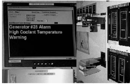
Figure 18.4. Responder monitoring system (photograph reproduced by kind permission of Compusult Ltd., Canada)
