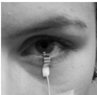
Figure 3.28. Gold foil ERG electrode in place
