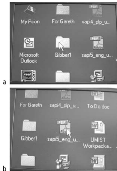
Figure 13.12a,b. Example of mouse movement. This shows the mouse pointer in a has been moved to the right in b . The display has scrolled to the right. The mouse pointer has centralised the image during the movement
