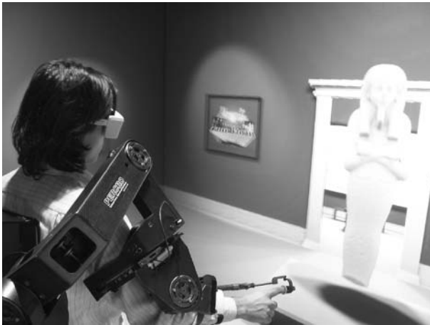
Figure 4.10. The Pure-Form display used together with a visual display in a museum. Image copyright Antonio Frisoli, Massimo Bergamasco, PERCRO, Scuola Superiore Sant'Anna, Pisa, Italy and used by permission
