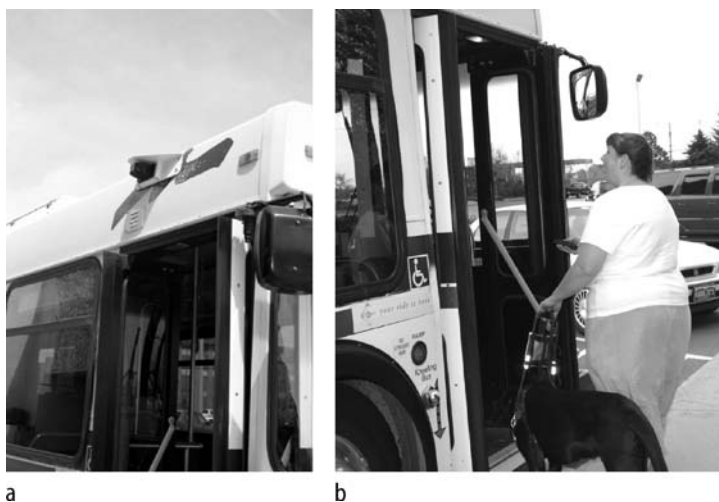
Figure 10.13a,b. Bus identifying system (photograph reproduced by kind permission of Mark IV Luminator, USA)
