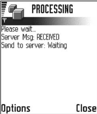
Figure 11.14. Screenshot showing that the bus stop server has received the requested bus number and the client is waiting for the bus
