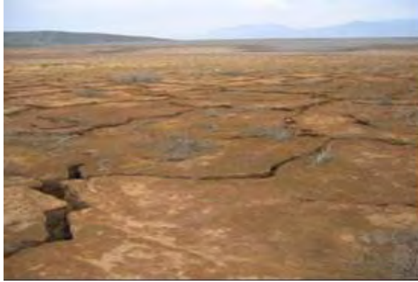
Fig.1 Desiccation cracks in uncovered tailings at Degmay.
