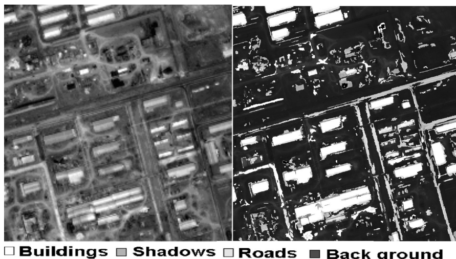
Fig. 11. (a) A part of the Esfahan Nuclear facility, Iran. (b) Classification result using minimum distance clustering
