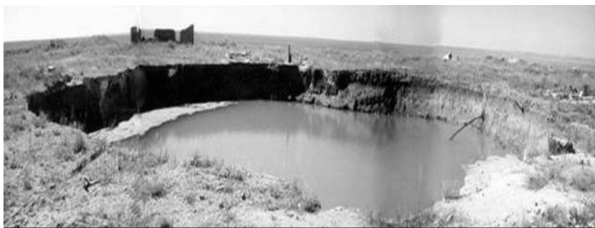
Fig.9. Collapse of the mine No. 3 after ground water rebound in N Kazakhstan.
