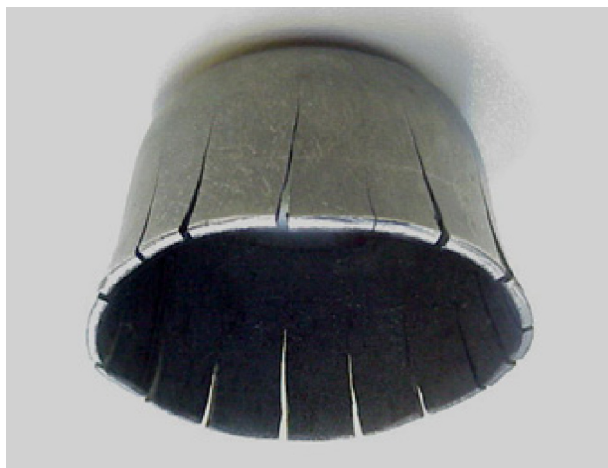
Fig. 10.15 Example of delayed fracture in deep drawn FeMnC TWIP steel.
