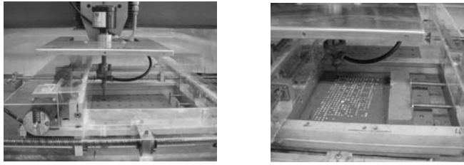
(a) Setting up the two-axis table on the waterjet machine tile on the table
