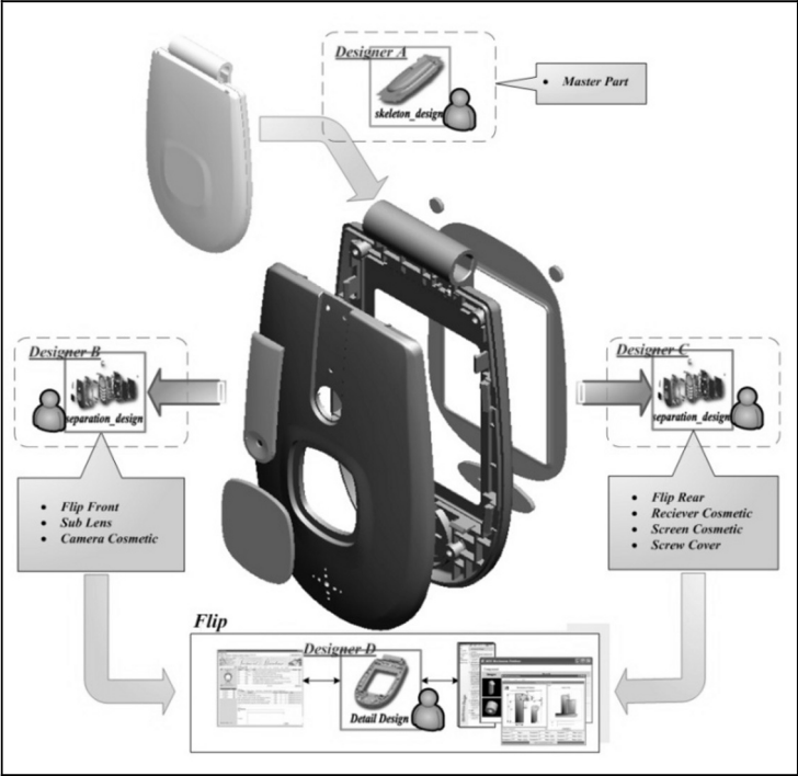
Figure 10. collaborative design of the cell phone component
