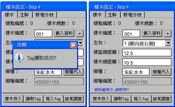
Fig. 6 Appearance picture of reading/writing tree RFID tag
