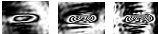
Fig. 6. Contour maps of phase difference digitally reconstructed from the sub-hologram
