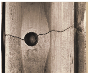
View of rivet hole A. No macro plastic deformation.
