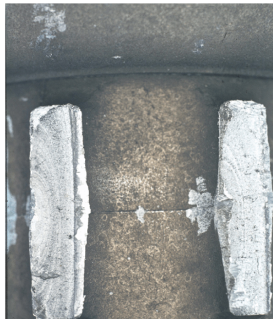
Fig. II.3 Two fracture surfaces with crack growth bands.
