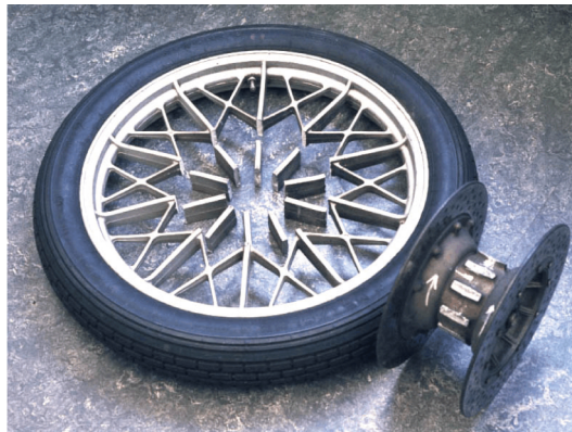
Fig. II.1 Wheel with 10 broken spokes and the disk brakes.
