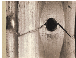
View of rivet hole B. Macro plastic deformation visible. Hole ovalization. Lateral contraction at right hand edge.
