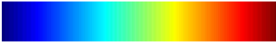
Fig. 1.3 In the cochleogram values are plotted using this color range. High values (relative to the maximum value to plot) are plotted in the colors on the right, low values (relative to the minimum value to plot) are plotted in the colors on the left). Values lower than the minimum value to plot are plotted in black; values exceeding the maximum value to plot are plotted in white.
