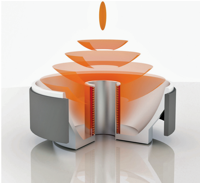
Fig. 38.7 Cylinder source. The electrical cylinder coil is covered by an insulation foil and a conducting membrane. The primary cylindrical wave is reflected and focused by a rotational parabolic reflector. The hollow center may be used for in-line fluoroscopic or ultrasonic stone localization
