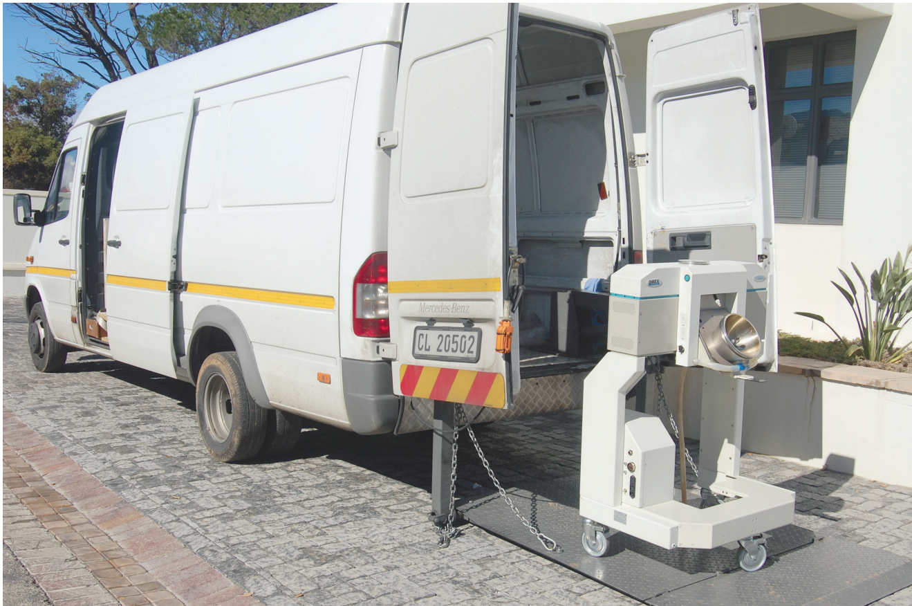
Fig. 107.1 Dedicated, safe, efficient transport with lifting equipment is needed to maintain a mobile SWL service
