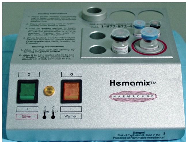
Fig. 52.2 Example of mechanical mixer required in the preparation of Tisseel
