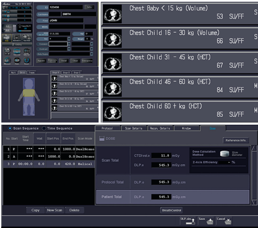
Fig. 14 Some screenshots from the user interface. The patient is registered from Modality Worklist (above, left), and there is an automatic selection of age-based protocols. Weight-based exam plans are available for pediatric applications (above, right). Detailed information about patient dose is available at all stages of the CT examination (below)
