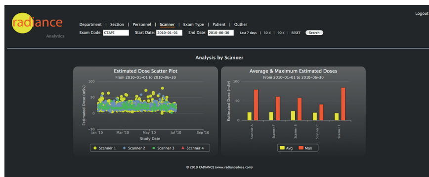
Fig. 5 The scanner dashboard enables comparison of dose estimates for a particular type of CT examination when obtained on different scanner models. Such an analysis is
