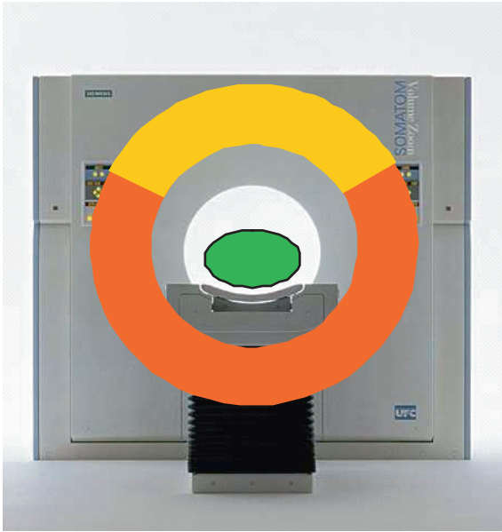
Fig. 6 Scheme of the X-CARE principle. Tube current is reduced substantially in the anterior part of the patient and slightly increases in the back of the patient
