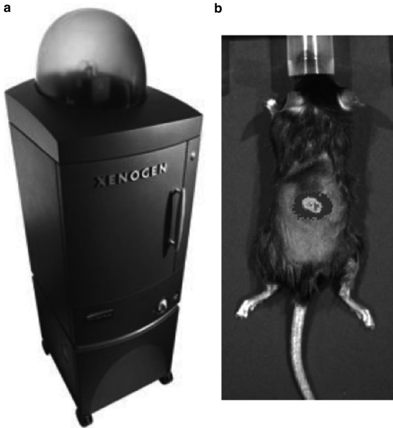
Fig. 2 Layout of the imaging system. (a) The IVIS molecular imaging systems (Caliper Life Sciences, Hopkinton, MA, USA). (b) A representative image of a mouse implanted with luciferase -expressing MSCs subcutaneously. Note the anesthesia mask in which the mouse nose is located, the area from which hair was removed, and the overlaid pseudocolor image
