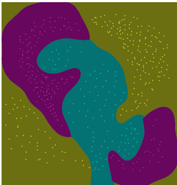
Fig. 16.3 SVM boundary for a three-class classification problem in two-dimensional space
