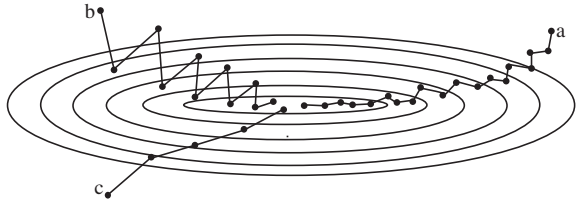
Fig. 4.2 Descent in weight space. a for small learning rate; b for large learning rate; c for large learning rate with momentum term added
