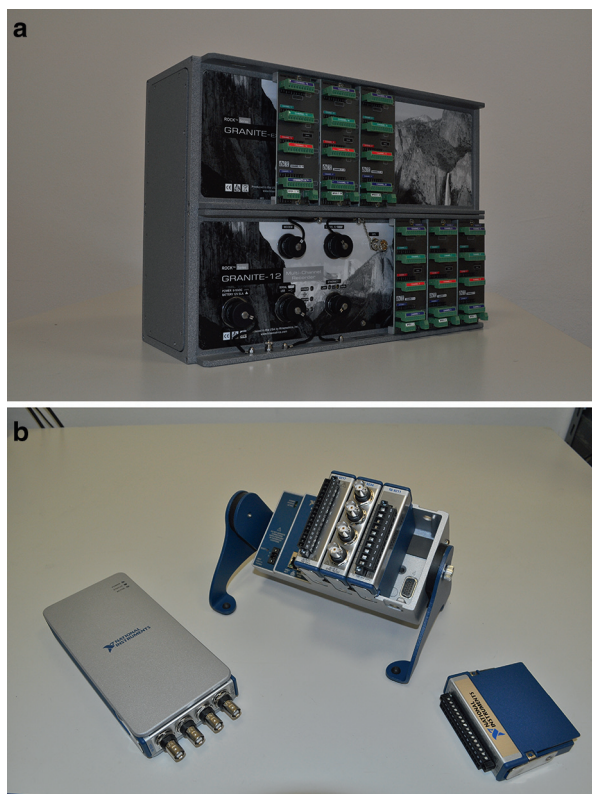
Fig. 3.6 Dynamic data acquisition system by Kinometrics Inc. (a) and programmable hardware by National Instruments™ (b)
