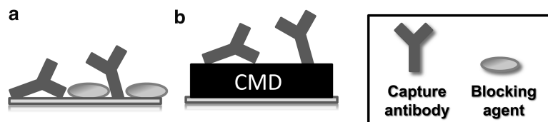
Fig. 1 Schematic illustration of capture antibody immobilization. (a) Standard ELISA based on the physical adsorption of capture antibodies (up to 14 h) and blocking agents (1 h) on polystyrene wells, and (b) modified ELISA involving the covalent attachment of capture antibodies (15 min) onto a carboxymethylated dextran (CMD) layer grafted on aminated wells
